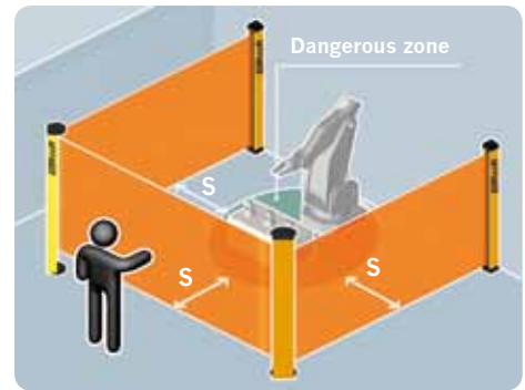
Three-side protection using deflection mirrors
