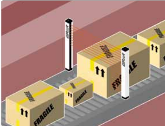
Measurement of the height of objects in transit on conveyor systems
